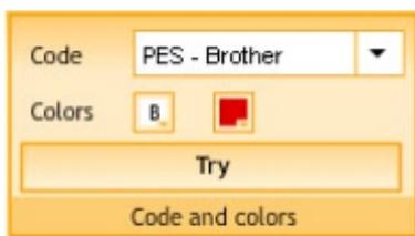
**Press the button TRY only once to generate the stitches and display a design pre-view.**
